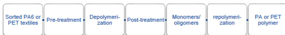
Figure 39 - General chemical recycling process of PET & PA6 (Duhoux T. & al, 2021)
