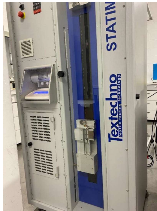
Figure 12 : Monofilament test: sample approaching its maximum elongation
